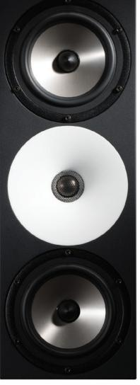
The Amphion speakers' MDF cabinets have no bass ports or venting holes for air to escape. Instead, they use an aluminum passive radiator located on the rear of the cabinet for low-end dispersion. This radiator is the same diameter as, and looks similar to, the low-frequency driver on the front. It is located on the same plane as the driver and moves perfectly in tandem to disperse and control low end.
