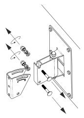
(5) Attach adjustable U-bracket to speaker adaptor-bracket using bolts (2), washers (2), and locknuts (2)
