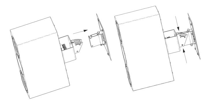
(7) Insert bolts (2), washers (2), locknuts (2), and locknut caps (2) to fasten adjustable U-bracket to wall-mount
