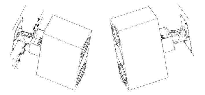
Set desired monitor tilt-angle (eg. 30 degrees pictured) and tighten adjustable hinge bolts
