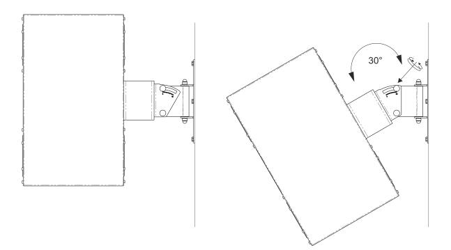
9 Adjust lateral monitor toe-in angle accordingly
