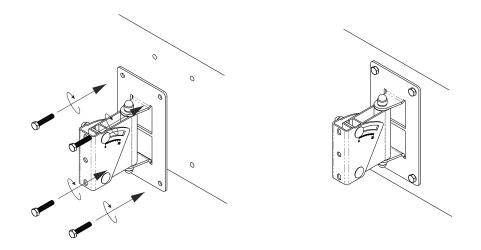
(4) Remove adjustable U-bracket from wall-mount ie. bolts (2), washers (2), locknuts (2), and locknut cap (2)
