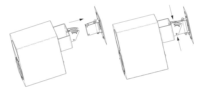
(7) Insert bolts (2), washers (2), locknuts (2), and locknut caps (2) to fasten adjustable U-bracket to wall-mount
