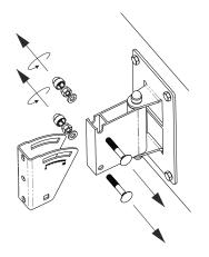
(5) Attach adjustable U-bracket to speaker adaptor-bracket using bolts (2), washers (2), and locknuts (2)
