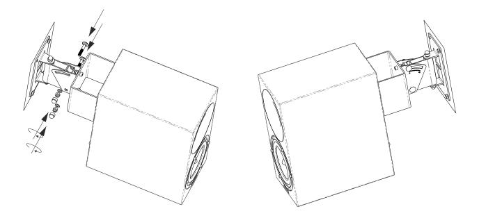
3) Set desired monitor tilt-angle (eg. 30 degrees pictured) and tighten adjustable hinge bolts
