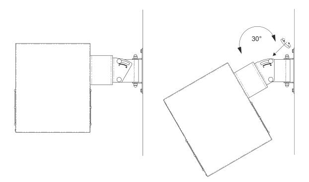
(9) Adjust lateral monitor toe-in angle accordingly
